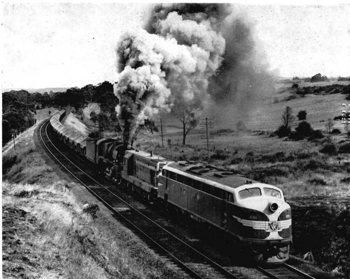
Steam and diesel locomotives combine to haul a heavy wheat train up the Warrenheip bank.
